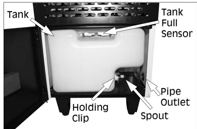
**NOTE:** The water tank full alarm will continually sound when the tank is removed and will not turn off until the tank is empty and correctly seated back in the machine.
