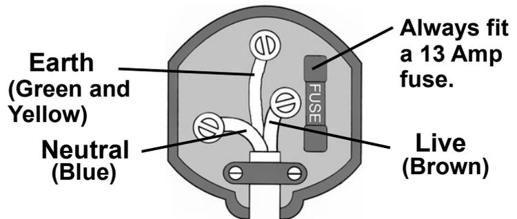
**Ensure that the outer sheath of the cable is firmly held by the clamp**
