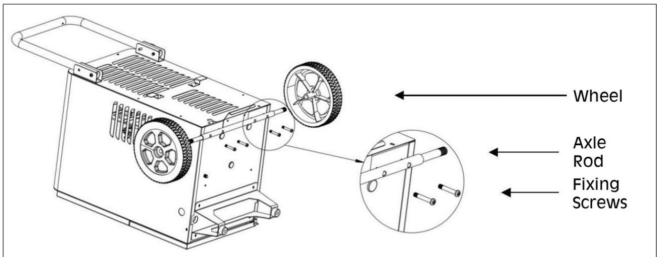
3. Once the wheels have been installed, place the machine in the upright position.
