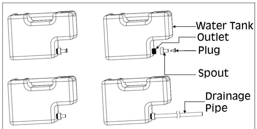
3. Place the end of the pipe onto the water tank spout and replace the tank back in the machine.
